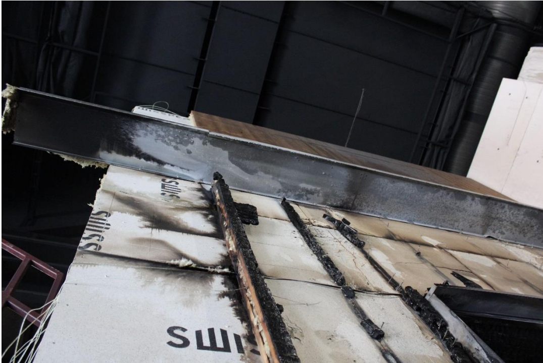
Photo No. 27 Test specimen after the test. Detailed photo below the second flame deflector.
