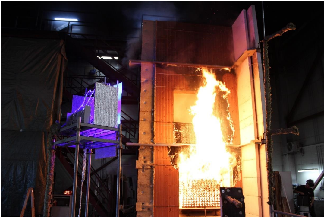
Photo No. 16 Test specimen 13 minutes into the test.
