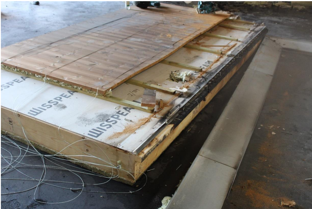
Photo No. 28 Test specimen after the test. Detailed photo of the top prefabricated cassette.
