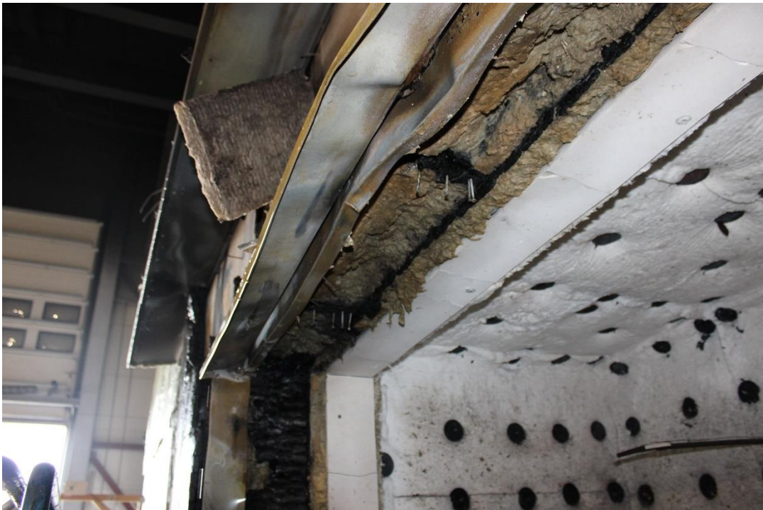
Photo No. 26 Test specimen after the test. Detailed photo of edge of burn specimen.
