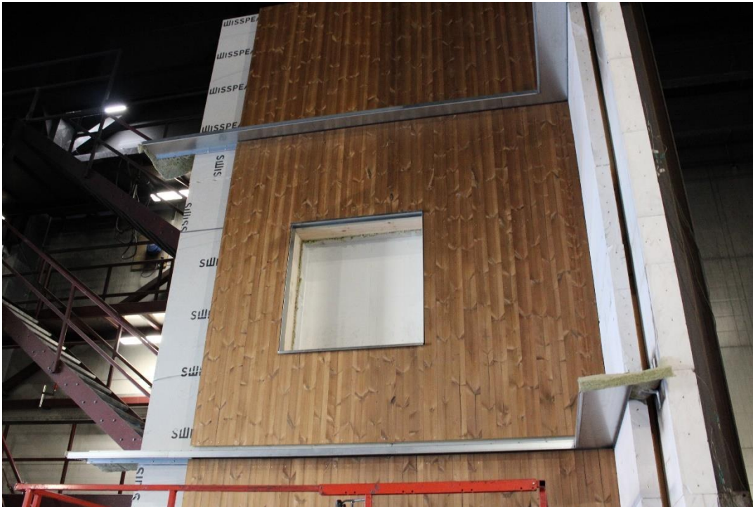
Photo No. 9 Vertical cladding mounting done. Insulation inside flame deflectors mounted.
