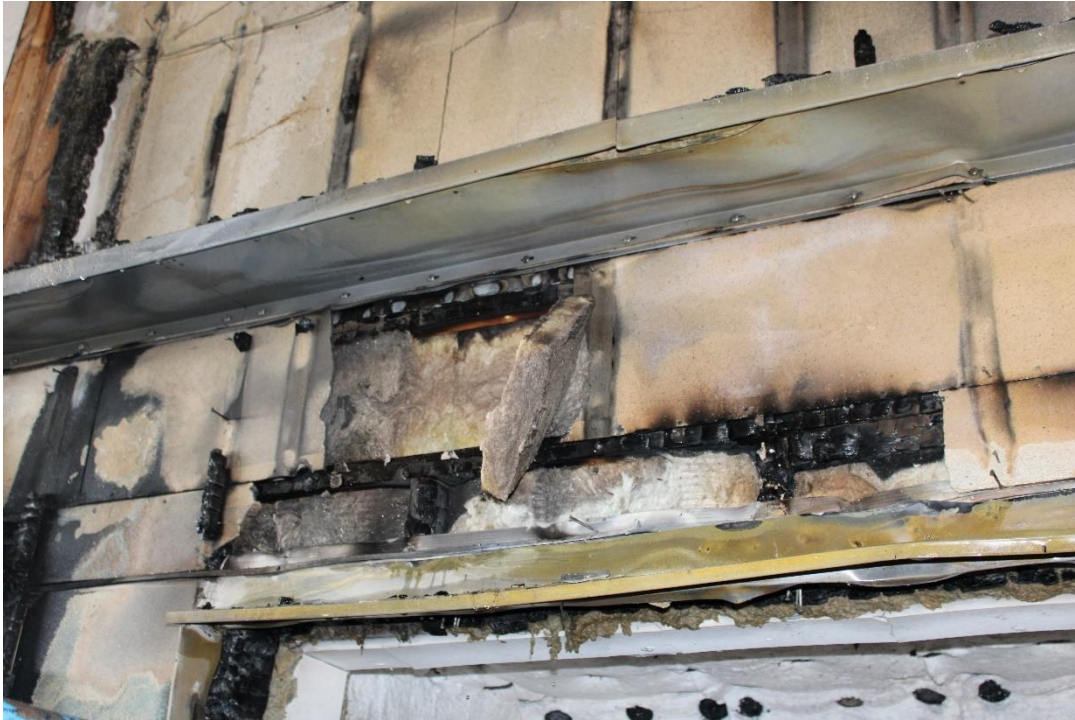
Photo No. 25 Test specimen after the test. Detailed photo below the first flame deflector.
